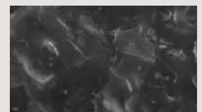
With Orevac® CA100 Homogeneous with matrix with embedded talc in PP
